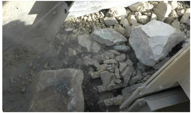
Adjustable grizzly openings provide some control over the size of material being fed into the crusher, as well as what is rejected ahead of the crusher. This saves crusher wear cost while boosting plant capacity.
