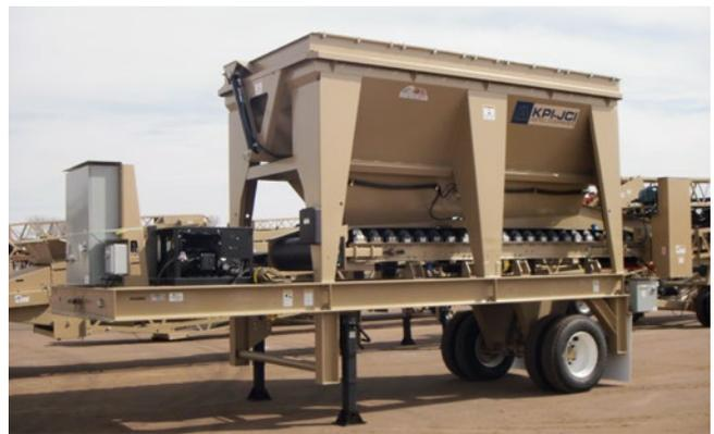
The biggest advantages of the roller belt feeder are their relatively low cost and that it is a “positive feed” device that does not rely on vibration to move material.
