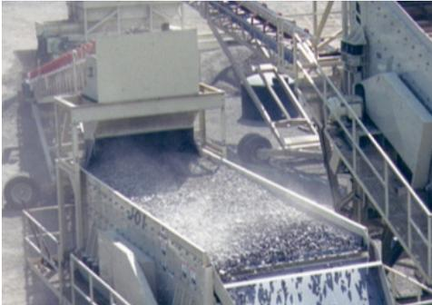
An 8x20 3-deck horizontal screen at the test facility
