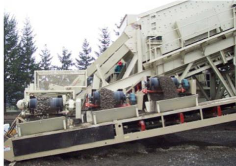
An 8x20 dual-shaft incline screen at the test facility
